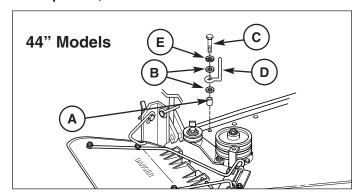
Figure 8. Install Belt Guide
